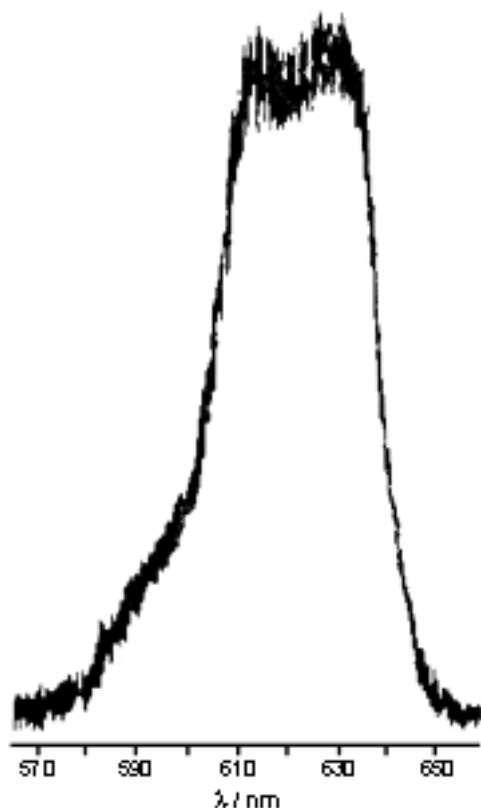
Fig. 1 Chemiluminescence spectrum taken during the reaction of 0.1 ml acetone with a solid mixture of 20 mg Curox and 17 mg \text{Eu}(\text{NO}_3)_3 at 90 °C.
