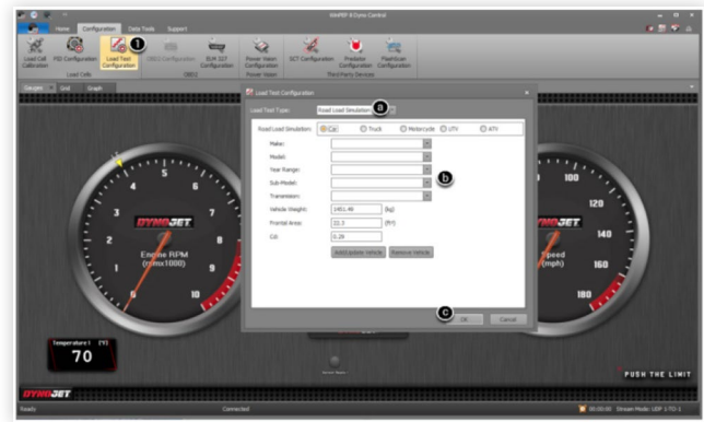
FIGURE 10 Road load control module configuration from chassis dynamometer manufacturer (dynojet-224xLC).
