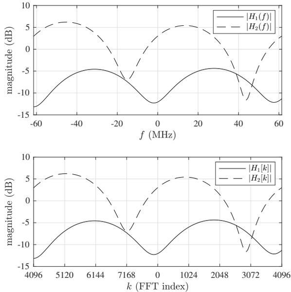
Fig. 2. The transfer functions of the two channels derived from orthogonally-polarized antenna elements in mobile handset. The first plot shows the channels as a function of frequency  $f$ . The second plot shows the channels as a function of FFT index.
