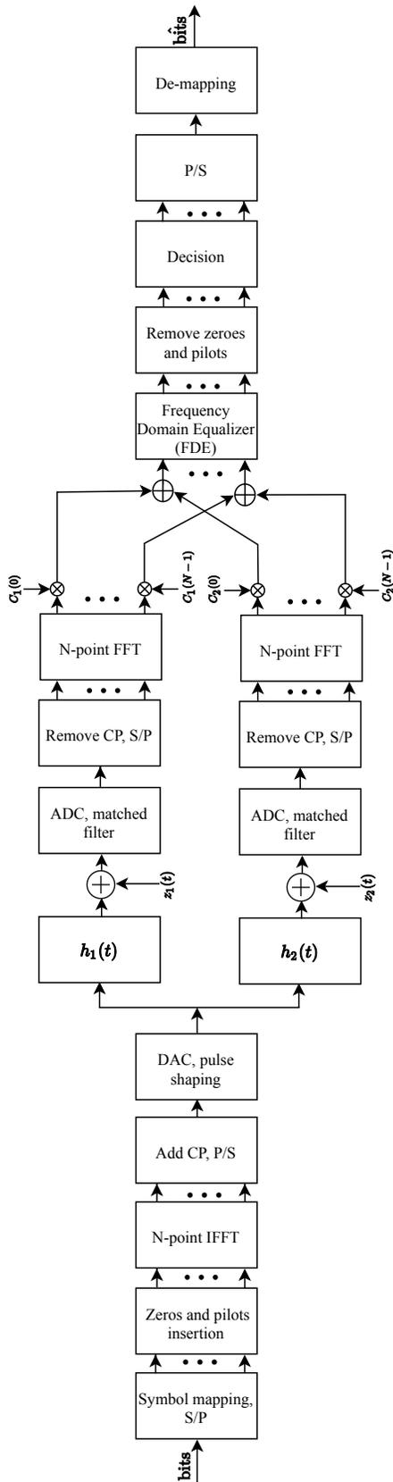
Fig. 3. Combine-then-equalize system architecture.
