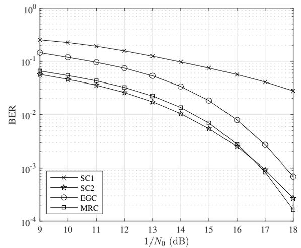
Fig. 6. The simulated BER performance of the equalize-then-combine system of Figure 4 for the four different combining techniques outlined in Section III-B.
