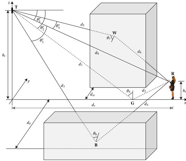
Fig. 1. An illustration of the 4-path multipath channel with polarization state information used in this paper.
