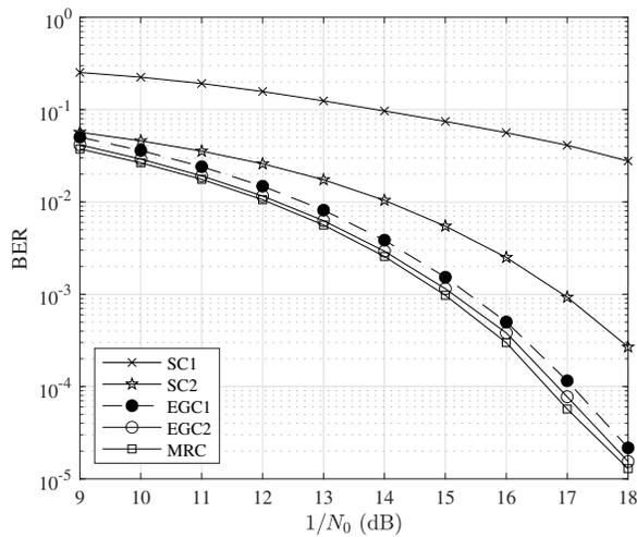
Fig. 5. The simulated BER performance of the combine-then-equalize system of Figure 3 for five different combining techniques outlined in Section III-A.
