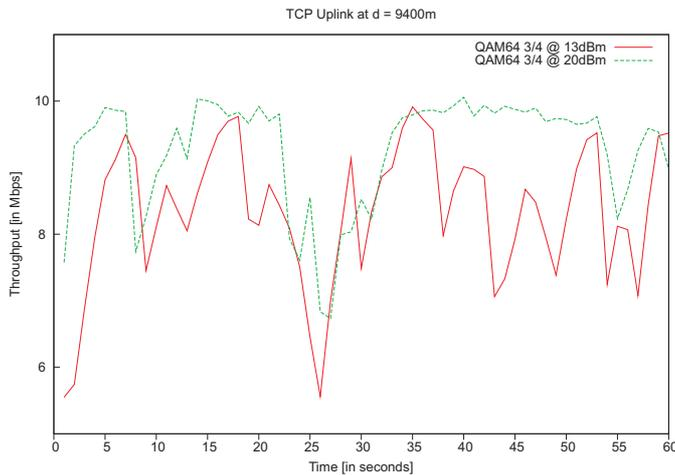
Fig. 5. Effect of Transmit Power
