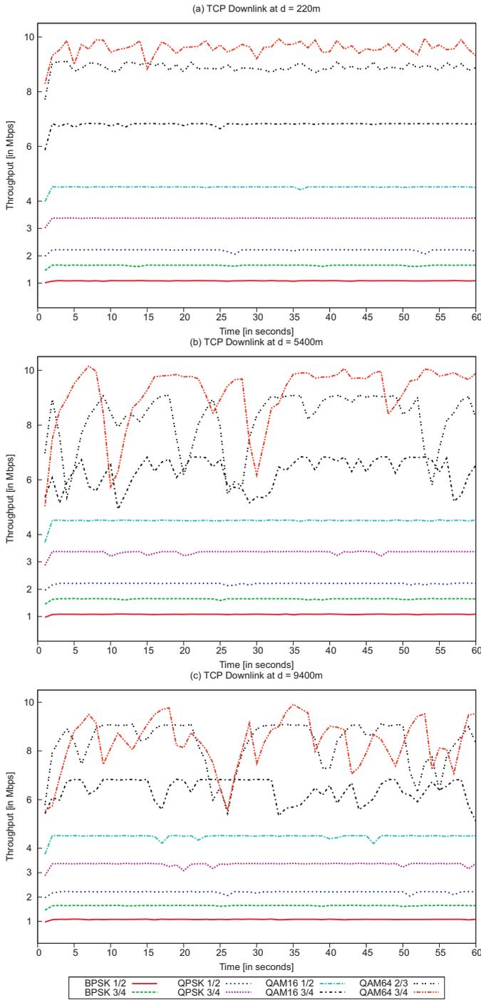
Fig. 3. TCP Downlink Throughput at  $d =$  (a)220m, (b)5.4km, (c) 9.4km
