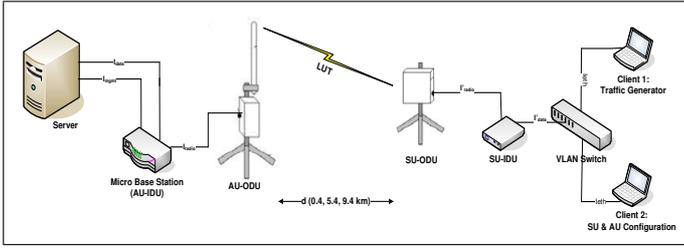
Fig. 1. Measurement Setup
