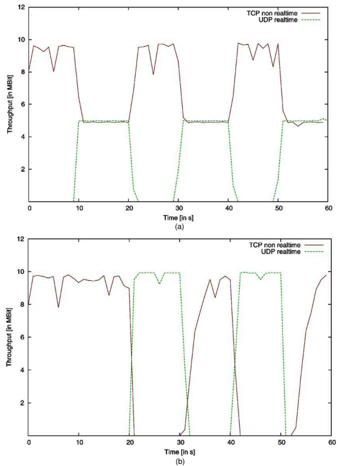
Fig. 4. QoS Measurement with (a) 5Mbps and (b) 10Mbps UDP traffic and TCP Background Traffic
