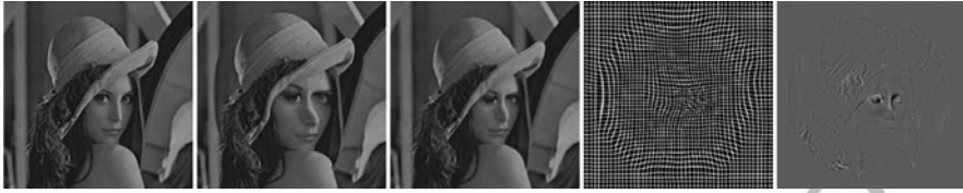
Fig. 9.8 FFD registration: from left to right – the reference, target, the registered target, deformation field, and error images
