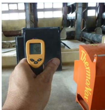
Figure 2. Infrared manual probe for surface temperature instant measurement.
