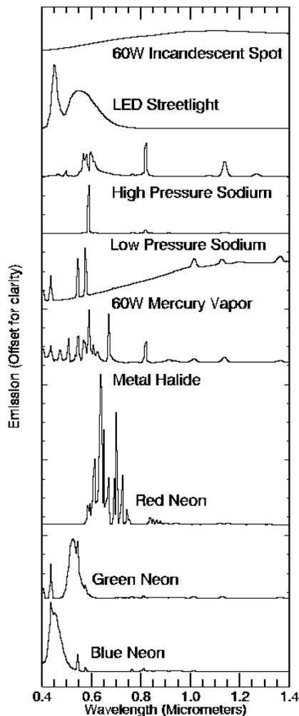
**Figure 2 - Comparison of VNIR/SWIR radiance spectra for selected night light types showing emission features. Spectra from the NOAA night-lights spectral library, measured with an Analytical Spectral Devices Spectroradiometer [3].**
