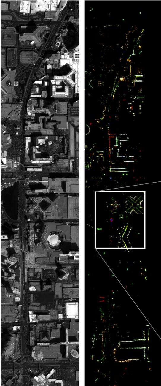
**Figure 3 – Left: Quickbird image at approximately 0.6m spatial resolution for a portion of the city of Las Vegas, NV. Right: True-color (0.65, 0.55, 0.45 micrometers as RGB) ProSpecTIR image covering the same area.**
