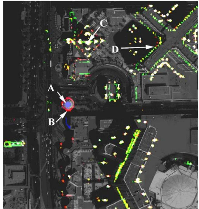
**Figure 6 - Night lights true color composite image overlain on Quickbird base. Note slight misregistration caused by non-nadir Quickbird view. These offsets could be corrected by orthorectifying both datasets with a high resolution DEM that included building models.**
