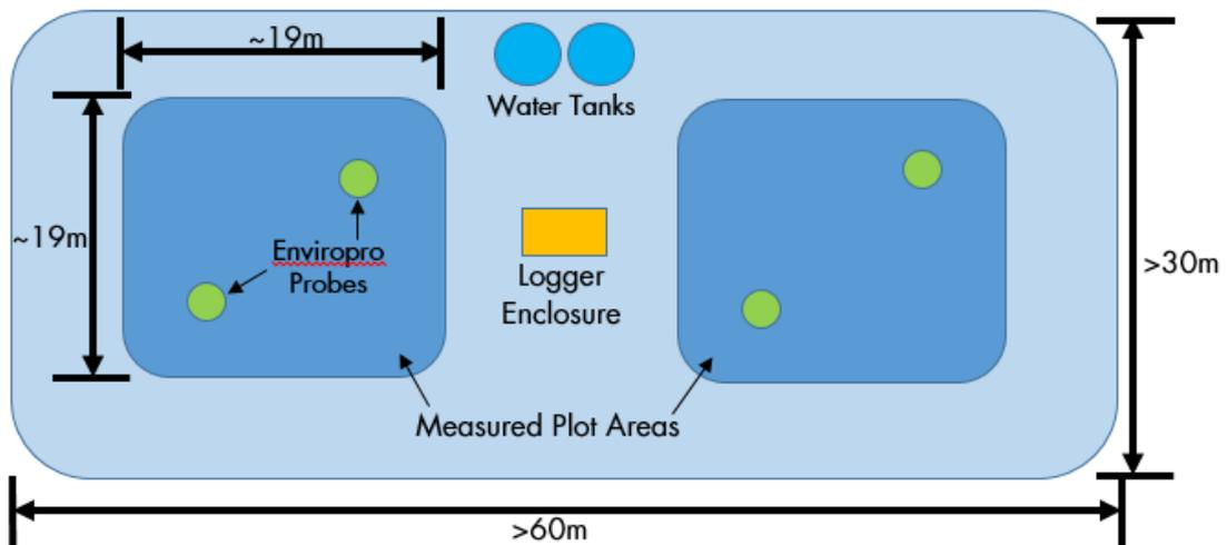
**Figure 1: Schematic drawing of plot configurations.**
