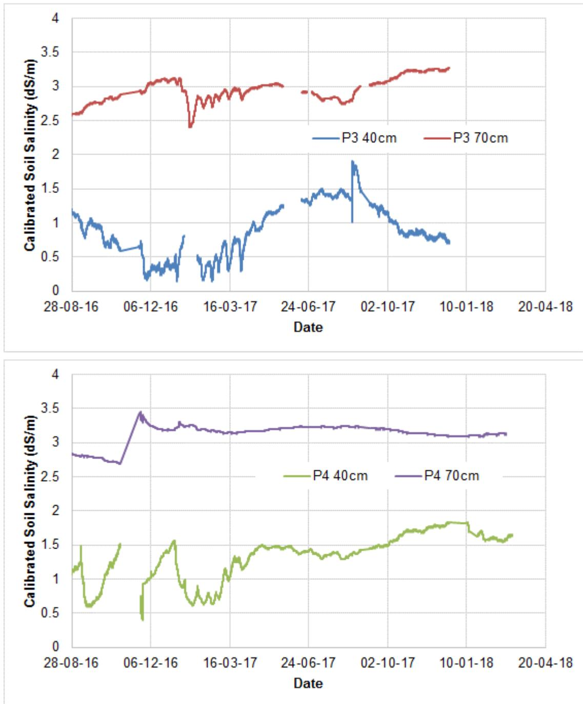
**Figure 9: Soil salinity for the thinner cover (0.5m) over the PAF waste dump at profile depths of 70cm, and 100cm. Probe 3 (top) and Probe 4 (bottom)**
