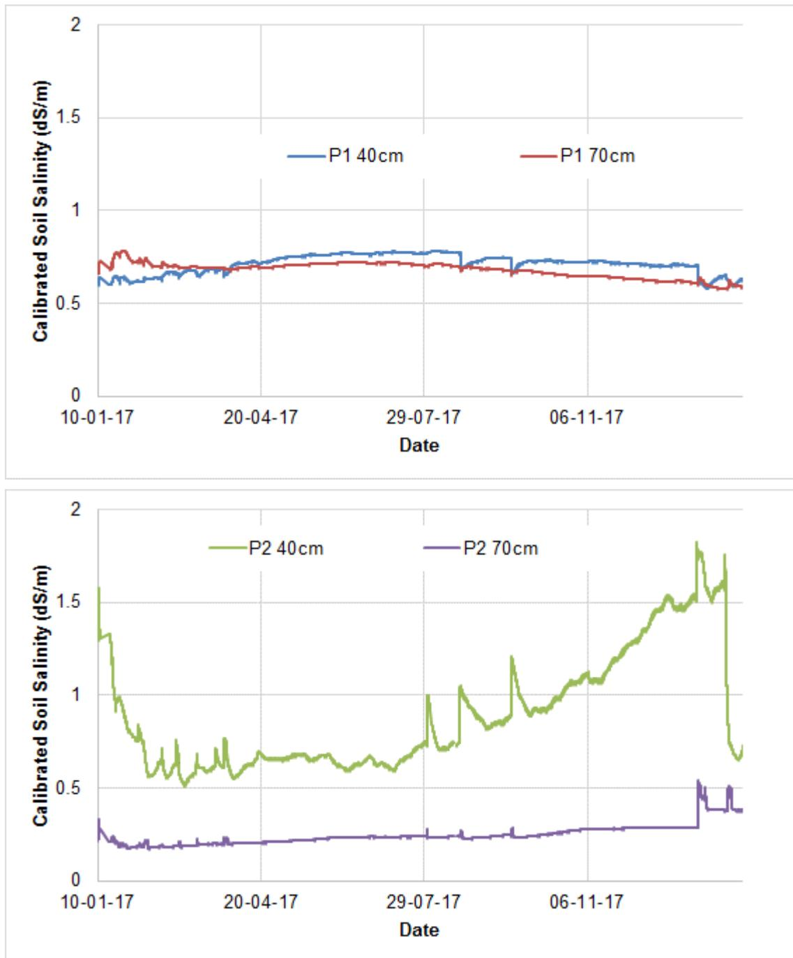
**Figure 5: Soil salinity for the thinner cover (0.4m) over the TSF at profile depths of 40cm and 70cm. Probe 1 (top) and Probe 2 (bottom)**
