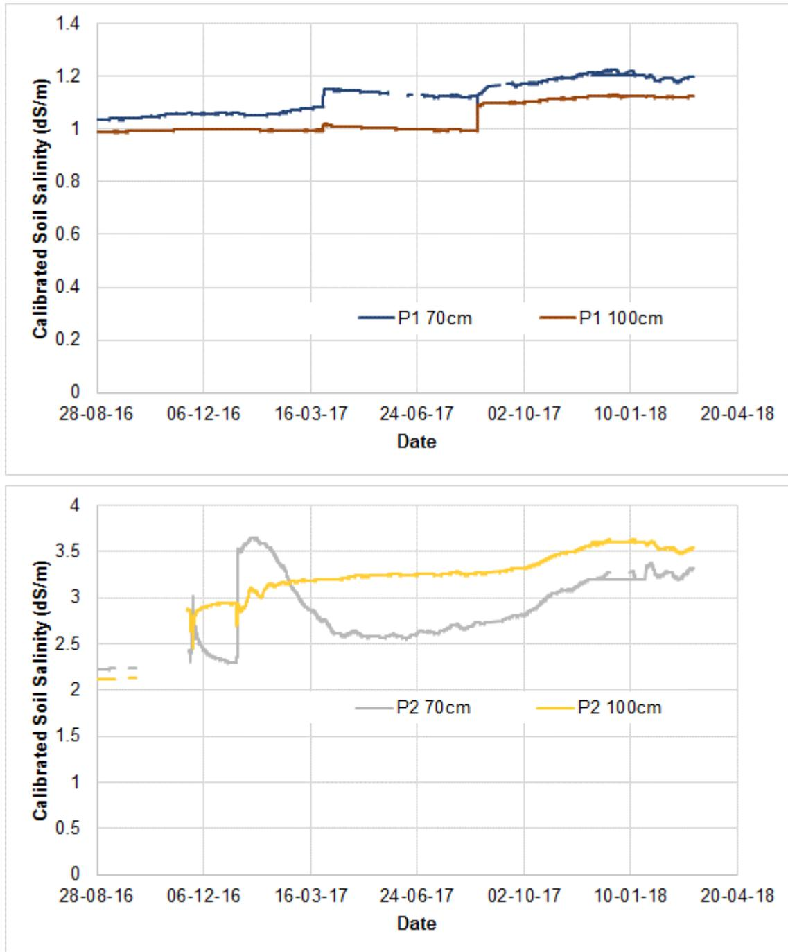
Figure 8: Soil salinity for the thicker cover (1.0m) over the PAF waste dump at profile depths of 70cm, and 100cm. Probe 1 (top) and Probe 2 (bottom)
