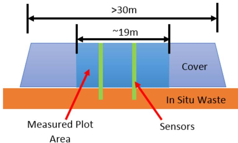
**Figure 2: Schematic drawing of Enviropro soil sensors installed through the cover layer and upper region of the underlying material.**
