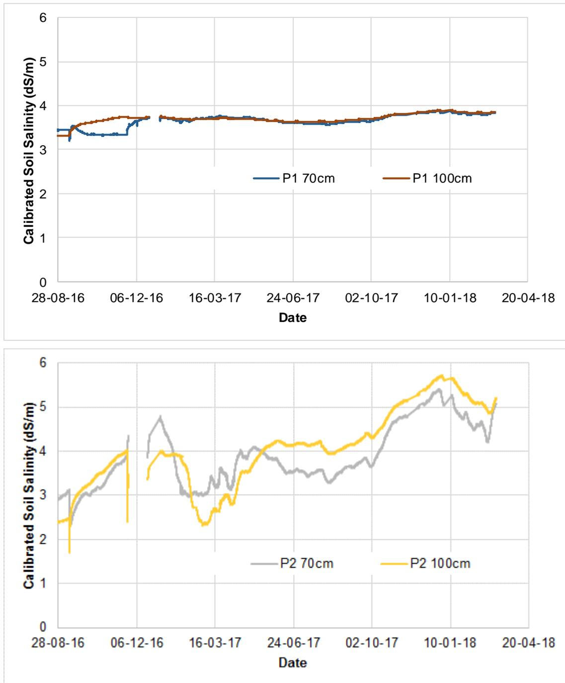
Figure 6: Soil salinity for the thicker cover (0.8m) over the heap leach pad at profile depths of 70cm and 100cm. Probe 1 (top) and Probe 2 (bottom)
