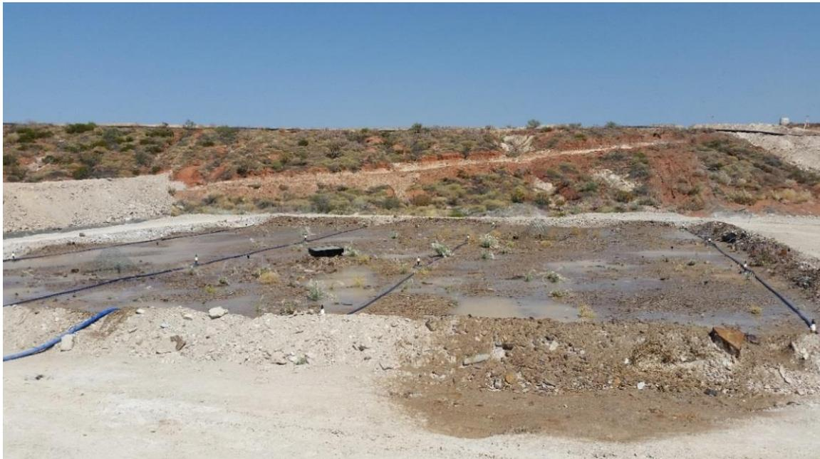
**Figure 3: Irrigation event using the portable irrigation system at the TSF**
