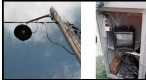
**FIGURE 1. Camera and TV/VCR Units Used in Data Collection**
