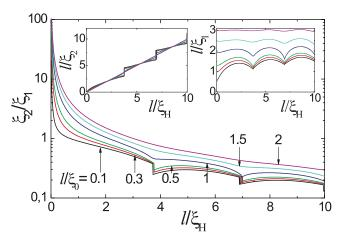
FIG. 5. (Color online) Dependence of the ratio  $\xi_2/\xi_1$  on inverse magnetic length  $l/\xi_H$  calculated for different ratios of  $l/\xi_0$ . Lefthand inset: Inverse decay length  $l/\xi_2$  vs inverse magnetic length  $l/\xi_H$  for different ratios of  $l/\xi_0$ . Right-hand inset: Inverse decay length  $l/\xi_1$  vs inverse magnetic length  $l/\xi_H$  for different ratios of  $l/\xi_0$ .
