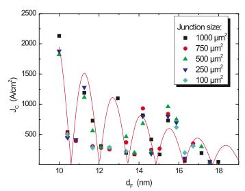
FIG. 4. (Color online) Critical current density of up to 60 single SIFS Josephson junctions against the *F*-layer thickness. The solid line indicates a theoretical fit after Eq. (1) with the two fitting parameters  $\xi_1$ =4.6 nm and  $\xi_2$ =0.45 nm.
