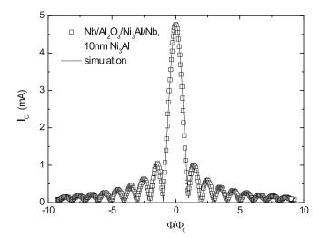
FIG. 2. Fraunhofer pattern of a typical circular Nb/Al/Al<sub>2</sub>O<sub>3</sub>/Ni<sub>3</sub>Al/Nb Josephson junction, measured at 4.2 K (rectangles). The junction size is about 1000  $\mu$ m<sup>2</sup>. The solid line results from a fit to the Fraunhofer function.
