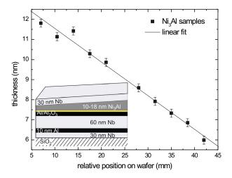
FIG. 1. (Color online) Ni<sub>76</sub>Al<sub>24</sub> film thickness measured at different positions on a 2 inch Si wafer with the RBS method. Inset, layer sequence in a cross section.
