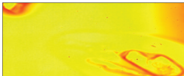
Picture 11. t.p on 142.9 °C, end crystal melting acetylsalicylic acid
