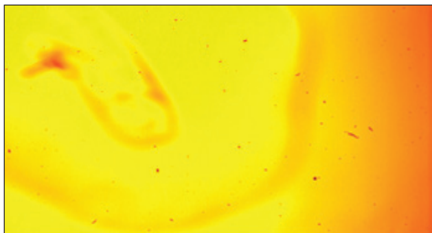
Picture 7. t.p. on 141.9 °C end of crystal melting acetylsalicylic acid
