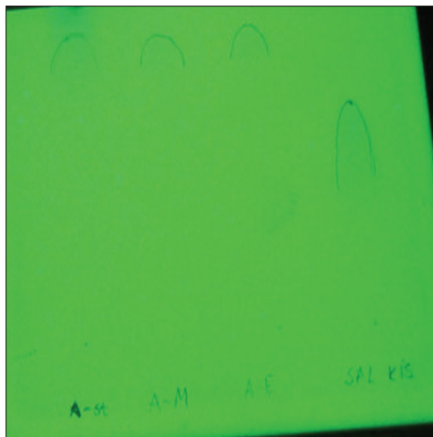
Picture 1. Plate HPTLC F 254 MERC with samples (aspirin–standard, aspirin–methanol, aspirin–ethanol and salicylic acid)
