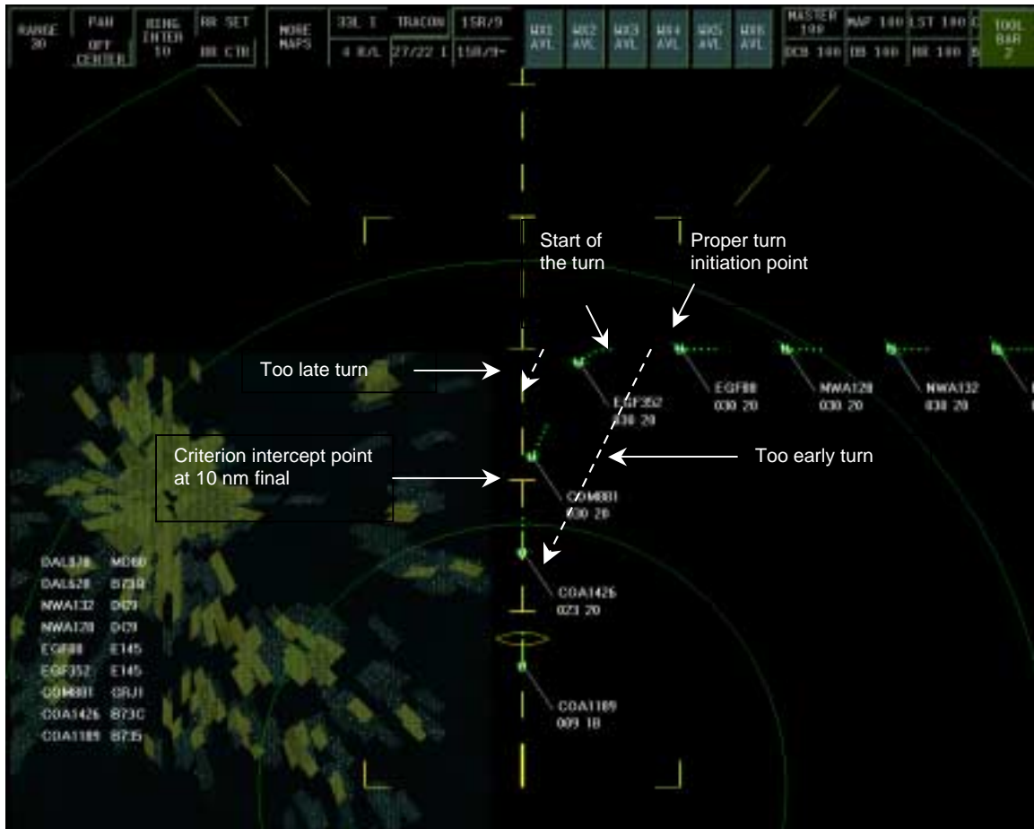
Figure 1. A screenshot from the experiment. Because the aircraft turning radius (which is a function of bank angle and speed), baseleg location, and intercept heading were constant, the point of final intercept was determined by timing of the turn initiation instruction (“[callsign] turn left heading 210, cleared for ILS runway 18 approach”) and subsequent delays in carrying out the instruction.
