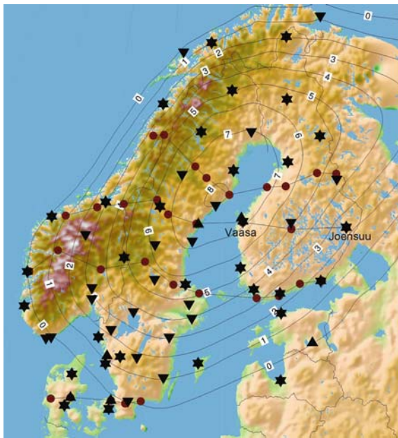
Fig. 1 GIA in Fennoscandia. Left: The upside-down triangles on the map are permanent GNSS stations, triangles stations where regular absolute gravity is measured as a part of the NGOS project, and dots with joining lines are the land uplift gravity lines, measured since the mid-1960s. Contour lines show the apparent land uplift relative to the Baltic mean sea level 1892–
