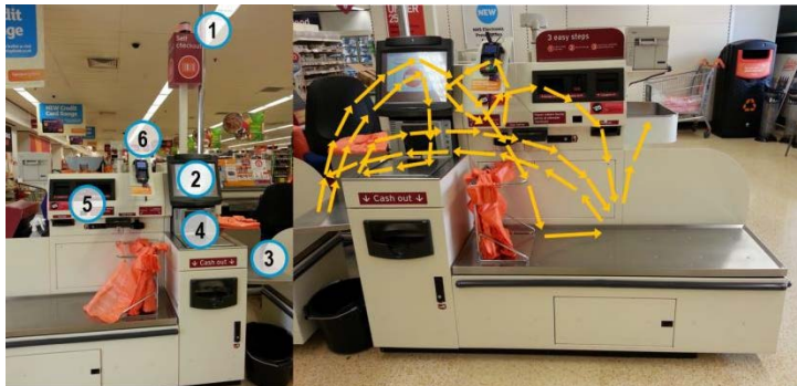
Figure 7 Self-Checkout System Outline (1. Lane light / Store attendant call / 2. Touch screen monitor / 3. Basket stand / 4. Barcode scanner and weighing scale / 5. Payment module / 6. ATM PIN pad)
