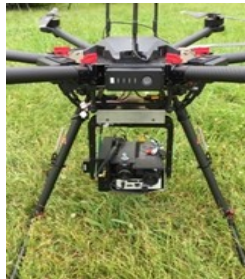
Figure 8. The ESCAPE payload, mounted to DJI M600 SUAS, featuring an EO FMV camera, an IR FMV camera and a SDR-based P-RF system with log periodic antenna.
