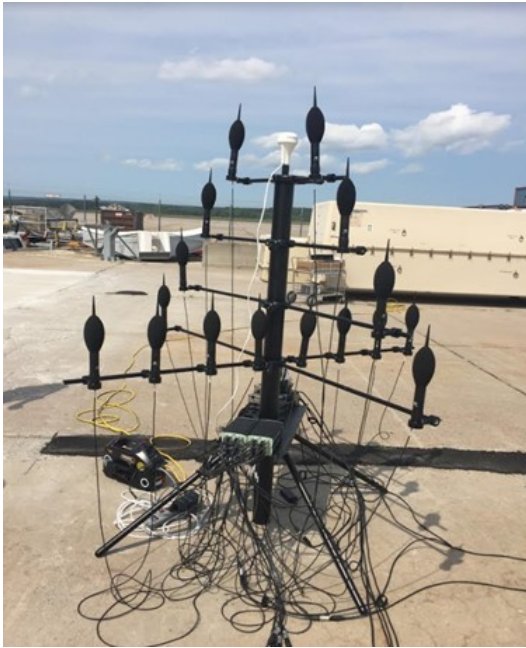
Figure 11. Acoustic array consisting of 16 microphones.
