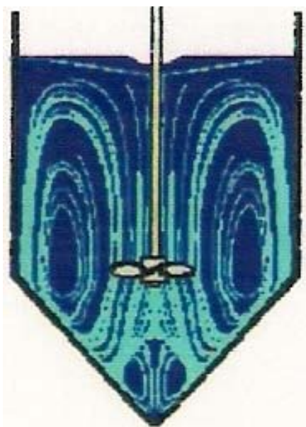
Fig. 9 Simulated flux lines in a conical bottom.
