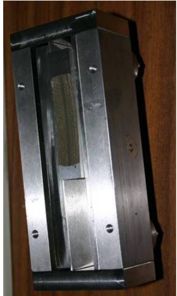
Fig. 4 Left: view of the 16 slices ready to be inserted on the cage-box for optical finishing. The reflecting side has been pre figured during the spark-erosion cut. The central piece is the spacer to be used only during optical finishing. Right: the slices and spacer inserted on the cage-box.
