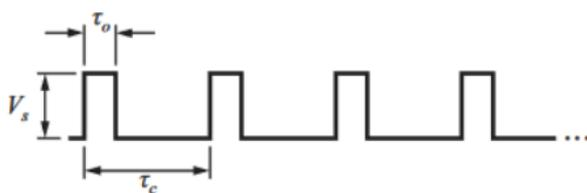
Figure 5: A pulse width modulated wave (Recktenwald, 2011)
