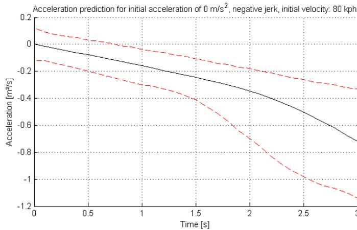
**Figure 7: Acceleration prediction for an initial velocity of 80 kph, an initial negative jerk and an initial acceleration of  $0 \text{ m/s}^2$ . The 2.5 percentile and 97.5 percentile are marked with the red dotted lines.**
