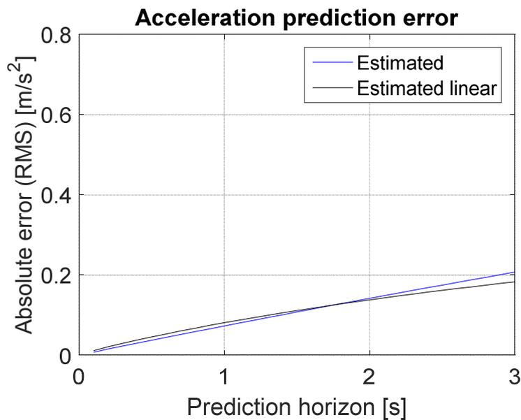
**Figure 9: Absolute error as a function of prediction horizon for constant driving ( $-0.5 \text{ m/s}^2$  acceleration  $< 0.5 \text{ m/s}^2$ ,  $n = 12301$ ). Current model in blue and simple linear extrapolation model in black.**
