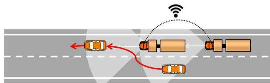
**Figure 1: Sharing information of surrounding traffic participants is desired to realize operational safety in combination with CACC.**
