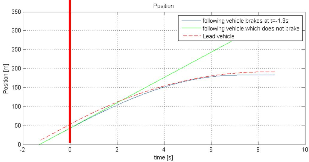
**Figure 5: Position of lead and following vehicle for 2 situations: following vehicle does not brake and following vehicle brakes at 1.3s before the braking action of the lead vehicle.**
