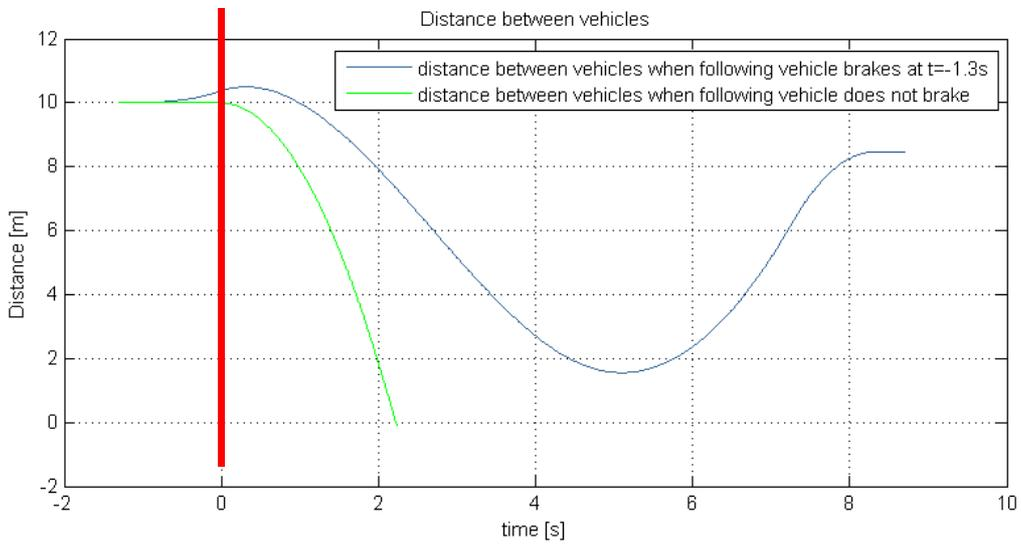
**Figure 6: Distance between lead and following vehicle for 2 situations: following vehicle does not brake and following vehicle brakes at 1.3s before the braking action of the lead vehicle.**
