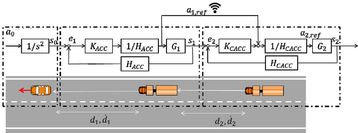
**Figure 4: Detailed description of use case 2a. The goal is to estimate  $a_{1,ref}$  such that in case the wireless link (temporarily or for a longer period) fails, the estimation can be used as a feedforward for the following truck. When  $a_0$  can be predicted for time interval  $t$ , given its history  $T$ ,  $a_{1,ref}$  can be calculated.**
