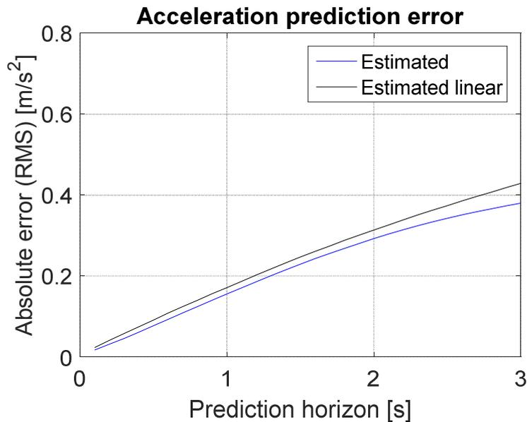
**Figure 11: Absolute error as a function of prediction horizon for braking events (acceleration < -1.0m/s<sup>2</sup>, n = 925). Current model in blue and simple linear extrapolation model in black.**
