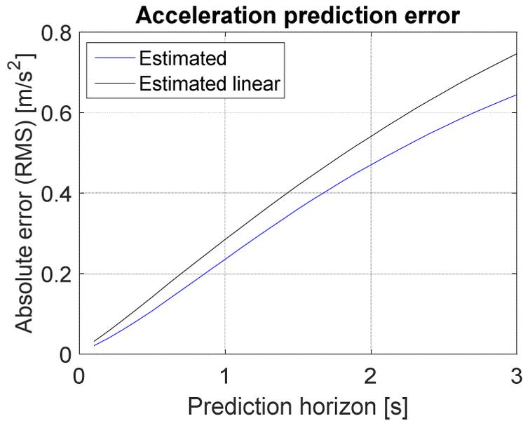
**Figure 10: Absolute error as a function of prediction horizon for acceleration events (acceleration > 1.0m/s<sup>2</sup>, n = 1315). Current model in blue and simple linear extrapolation model in black.**
