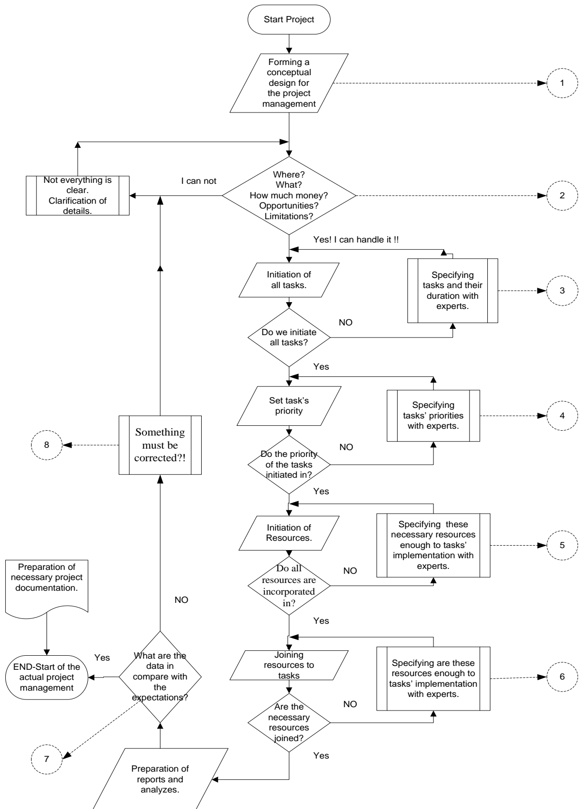
Graph 1. Algorithm for work in the management of projects using software tools
