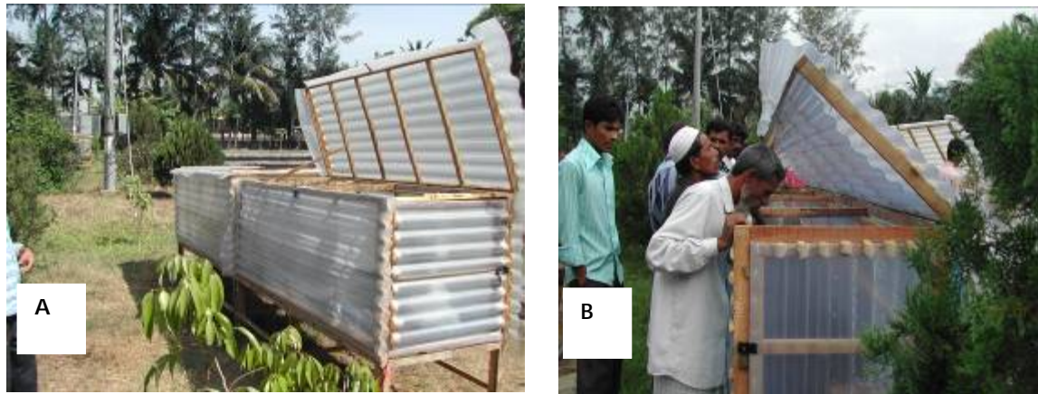
Fig. 3. Picture showing, (A) single layer, (B) double layer construction of the transparent model dryer usable in the presence as well as in the absence of the sun.
