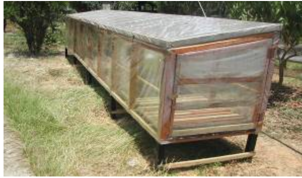
Fig. 5. Picture showing a complete 18 feet BFRI Fish Dryer covered with 0.2 mm transparent celluloid
