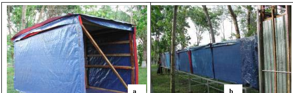
Fig. 1: A single unit of the emergency dryer (7'x3.5'x3.5')
