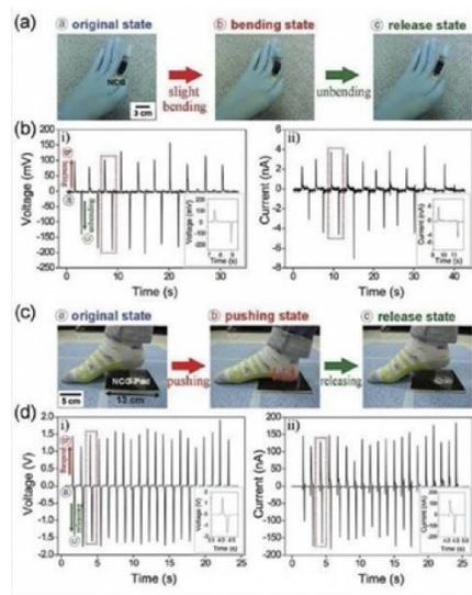
Figure 2. (a) a small-scale nanocomposite generator ( $4.1 \times 5.1 \text{ cm}^2$ ) bent and released by a human finger; (b) display of output voltage and current signals due to human finger movement; (c) a large-scale nanocomposite generator (with an area of  $13.13 \text{ cm}^2$ ) is shown; (d) Generating voltage and current signals due to foot movement [18].
