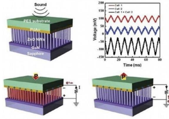
Figure 6. Generation of potential and output current in a Nano generator due to sound waves hitting zinc oxide nanowires [38].
