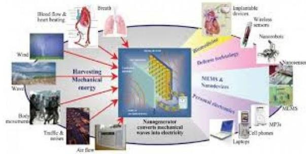
Figure 1. Scheme of electric current generation by a piezoelectric Nano generator based on zinc oxide nanowires by absorbing the mechanical energy of the environment and also a view of the potential applications of Nano generators for the future [16].
