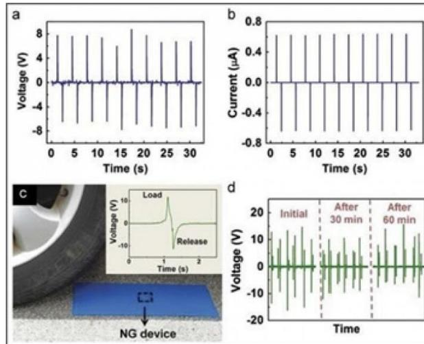
Figure 4. Energy collection by passing car tires through the Nano generator; (b), (a), and (d) represent the output voltage and current signals, and (c) represent the moment the tire passes through the Nano generator [33].
