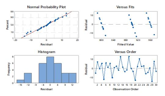
Fig. 1: Residual plots of the austenitising temperature model
