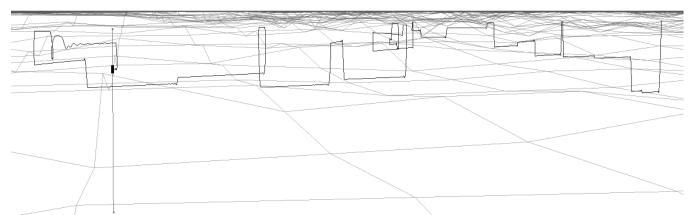
Figure 3: A screenshot of the simulation GUI, showing the position and history of a float over approximately 48 hours. The float's vertical position is indicated by a line connecting the surface to the sea-bottom.
