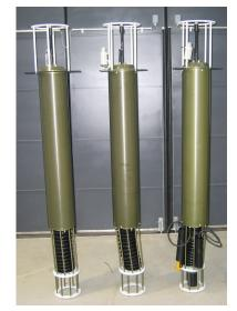
Figure 2: Three SWARM floats, ready for testing
