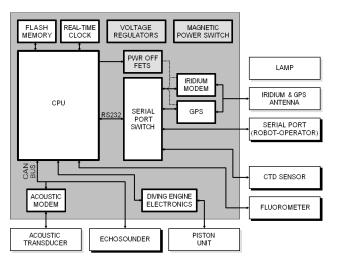
Figure 1: Block diagram of SWARM float subsystems
