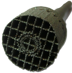
FIGURE 1.7 Shaft with the support material that needs to be removed
