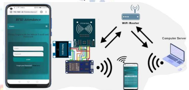
Figure 3: IoT based RFID Attendance Monitoring System using ESP32
