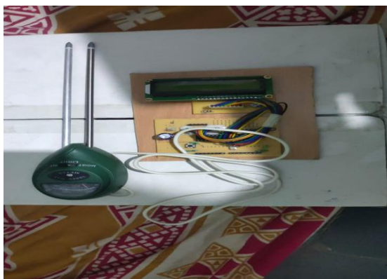
Fig:5. Set-Up of TDS
