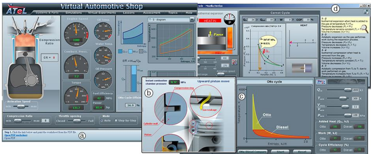
Figure 4. The virtual experiment “Influence of Compression Ratio on Engine Operation Cycle” performed at the v-Lab “Internal Combustion Engine Design and Operation”
