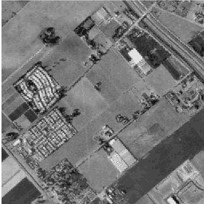
Figure 15: Image compressed at 0.46 bpp using a compression/classification encoder.
