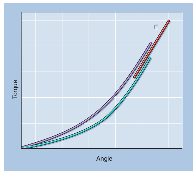
FIGURE 9.2 Schematic of a torque-joint angle plot during repeated passive stretches of a muscle group. Stress relaxation makes the passive torque at a given joint angle in subsequent stretches (blue line) less than in the first stretch (purple line). The stiffness (E) of the muscle group in these stretches, however, is not different.
