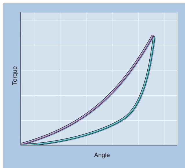
FIGURE 9.3 Schematic of a torque-joint angle plot of the elongation (purple) and restitution (blue) phases of a passive stretch of a muscle group. The energy lost (hysteresis) is the area of the loop between the loading and unloading phases.
