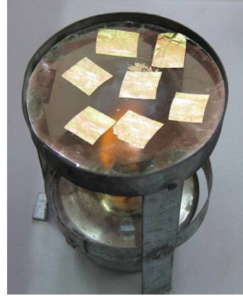
Figure 17.3 Bulk annealing: Gold foils placed on a mica tray over the flame.
