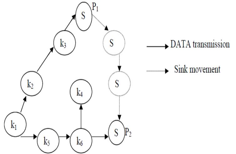
Figure 2: Data transmission with mobile sink
