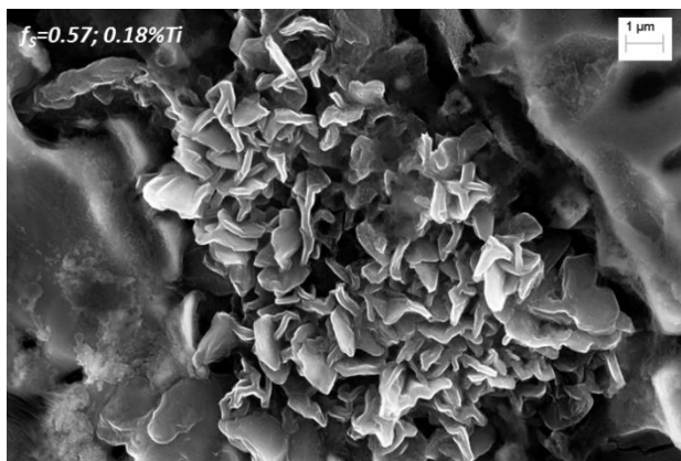
Fig. 9. Deep etching SEM images of iron Q2SIG (0.011% S, 0.32%Ti).
