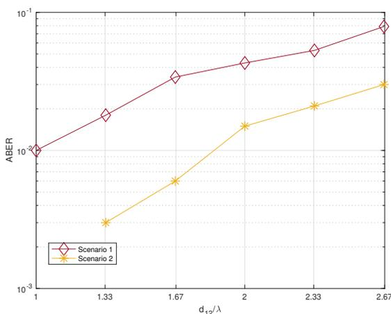
Figure 6: ABER of the Noncoherent ML detector versus  $d_{12}/\lambda$  for scenarios 1 and 2 and ternary constellation.
