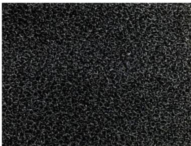
Figure 1: Porous carbon foam material used as interface medium in experiments
