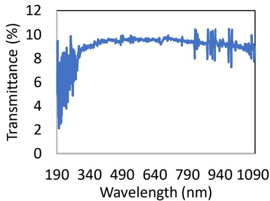
Figure 2: Optical transmittance of Carbon Foam interface medium, measured with GENESYS 10S UV-Vis Spectrophotometer
