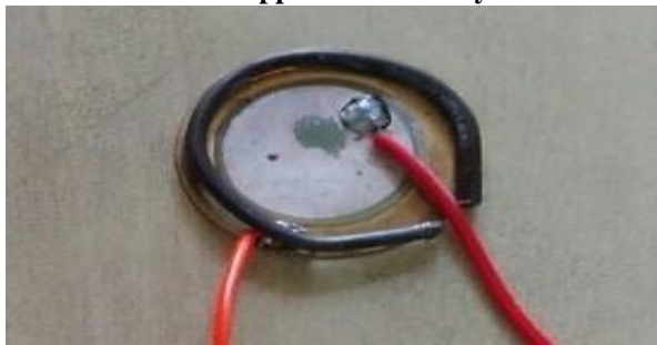
Figure 7. Piezo patch with circular supported boundary condition
