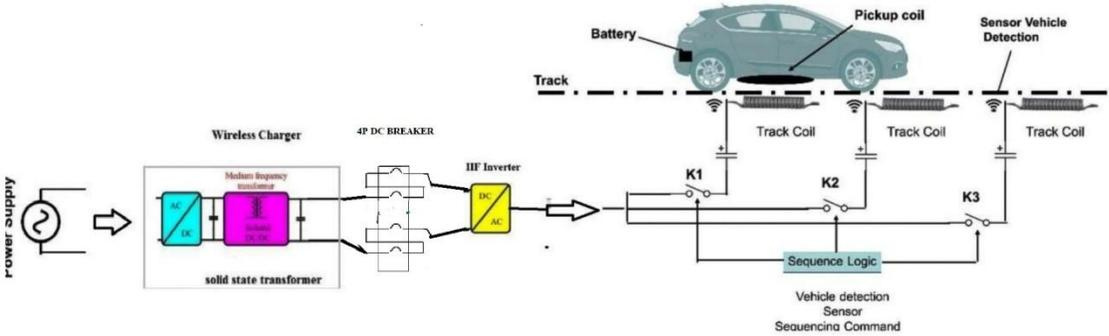
Fig.10 .SST based dynamic charging with 4P DC breaker.[12]
