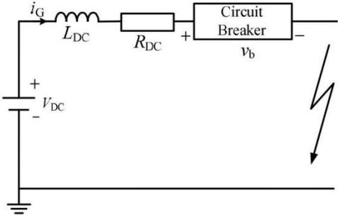
Fig.1. DC Breaker equivalent circuit [1]
