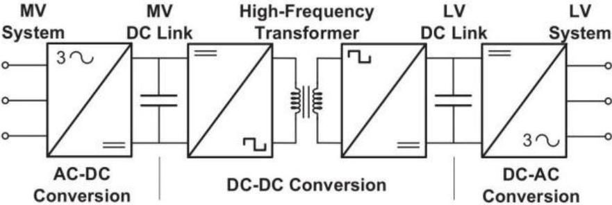
Fig. 2. The solid state transformer's block diagram [3]
