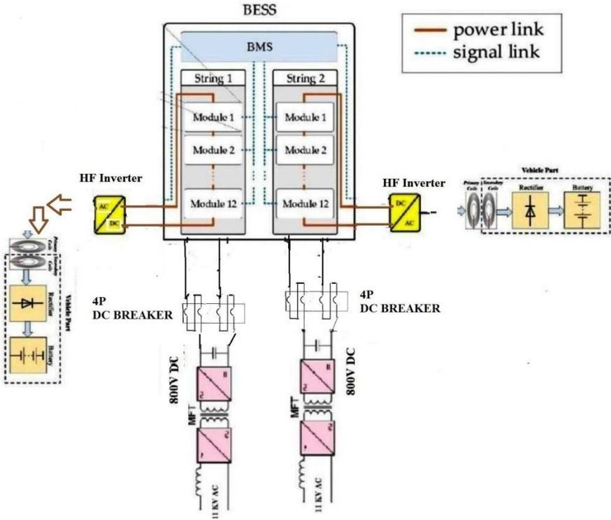
Fig.9.SST based wireless charging with 4P dc Breaker[11-12]
