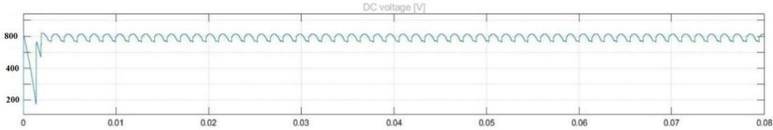
Fig. 7. DC output voltage of SST[9]
