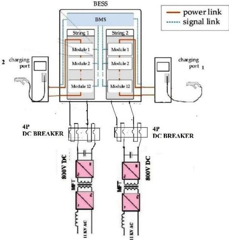
Fig .8. SST Based conductive charging with 4P DC breaker[11]
