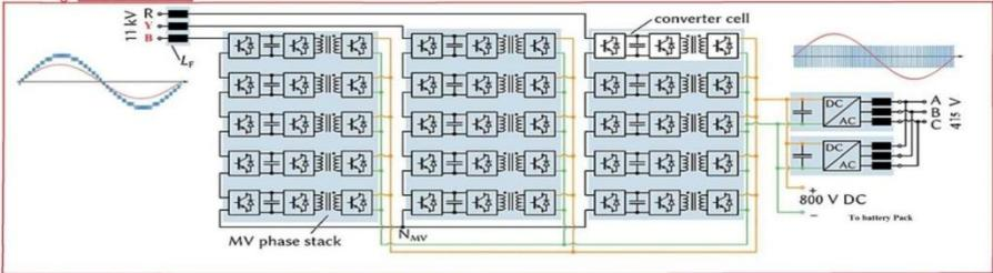
Fig. 6. circuit topology of SST.[10]
