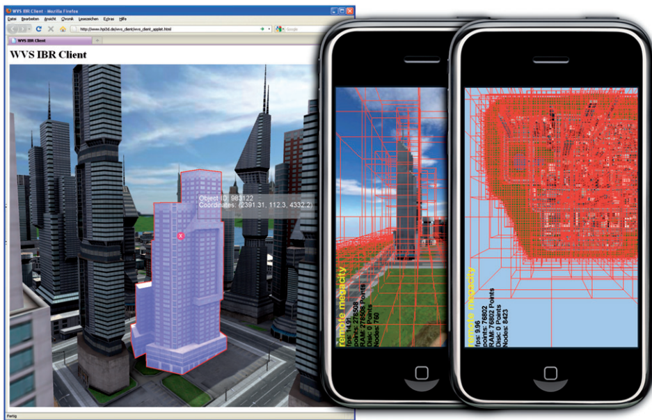
Figure 4. Left: Screenshot of a web-based WVS IBMR client application (Section 5.2) executing inside a web browser. The IBMR client shows a highlighted and annotated feature that was selected by the user. The IBMR client represents the remote 3D GeoVE locally as sets of 3D depth triangle meshes. Middle, right: Screenshots of a WVS PBMR client application (Section 5.3) executing on the smartphone Apple iPhone. The screenshots depict a close up view of a 3DGeoVE (middle) and an overview (right). The PBMR client represents the remote 3D GeoVE locally as an octree that contains 3D surface patches in nodes and leafs. In the screenshots, the client draws the bounding box of each octree node traversed in the rendering algorithm to illustrate the underlying hierarchical spatial data structure.
