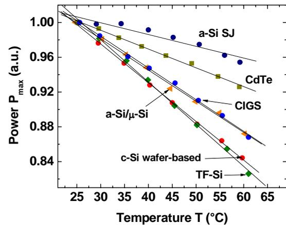
**Figure 2:** Modules' maximum power  $P_{max}$  as a function of the temperature for the different technologies under test. The values are normalized to STC values to facilitate a fair comparison between different technologies. Linear fits to these data provide the relative temperature coefficients for  $P_{max}$  ( $\gamma_{rel}$ ).
