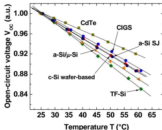
**Figure 3:** Modules' open-circuit voltage  $V_{oc}$  as a function of the temperature. The values are normalized to STC values. Linear fits to these data provide the relative temperature coefficients for  $V_{oc}$  ( $\beta_{rel}$ ).
