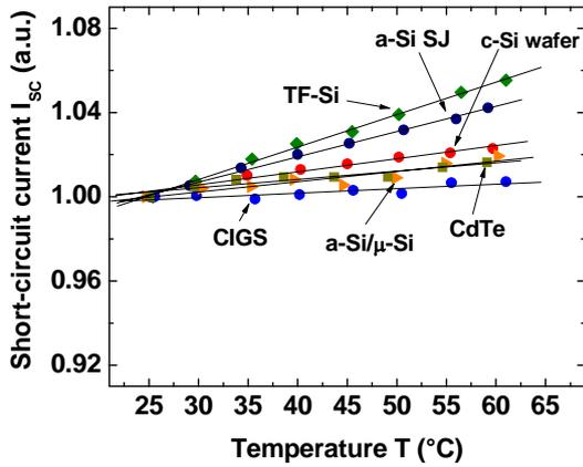
**Figure 4:** Modules' short-circuit current  $I_{sc}$  as a function of the temperature. The values are normalized to STC values. Linear fits to these data provide the relative temperature coefficients for  $I_{sc}$  ( $\alpha_{rel}$ ).
