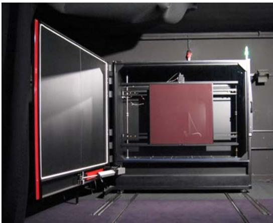
**Figure 1:** The thermostatic chamber used to realize temperature coefficient (TCO) measurements of the thin film devices.
