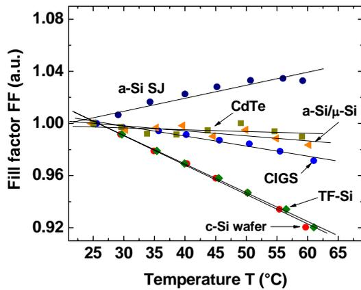
**Figure 5:** Modules' fill factor FF as a function of the temperature. The values are normalized to STC values. Linear fits to these data provide the relative temperature coefficients for FF ( $\kappa_{rel}$ ).
