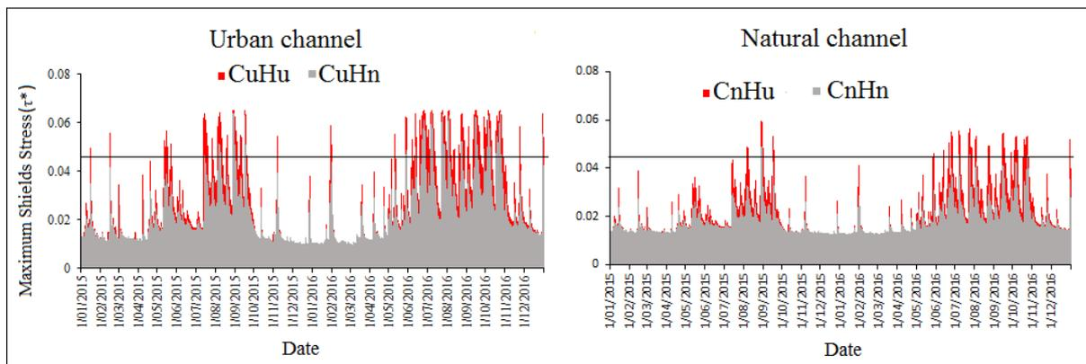
Figure 2. Daily maximum Shield stress for the two study sites for each modelled scenario. Solid horizontal black line show the critical Shields stress for bed particle mobilization ( $\tau_c^* = 0.045$ ).
