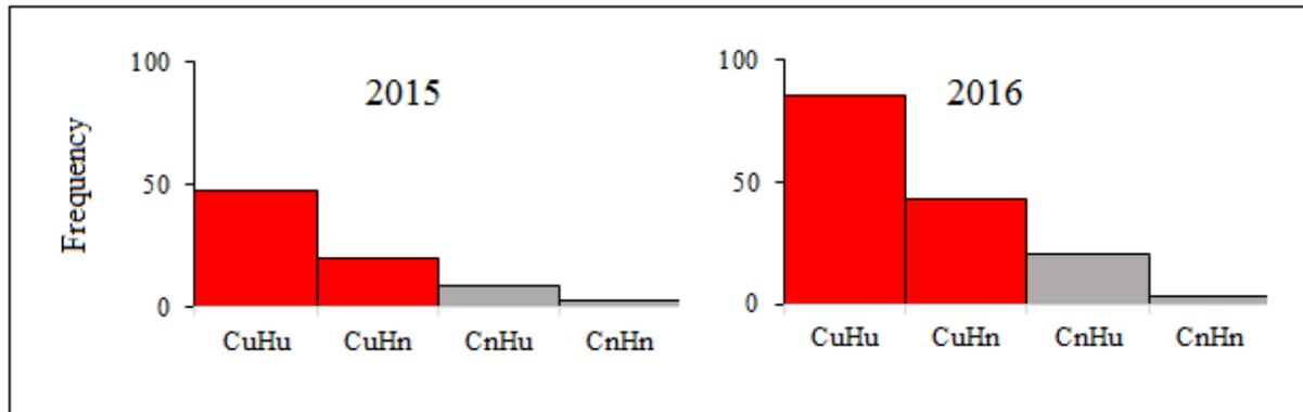
Figure 3. Number of days Shields stress was above critical threshold of the modelled scenarios during the study period. Red and Grey indicate scenarios in the urban and natural channel respectively.
