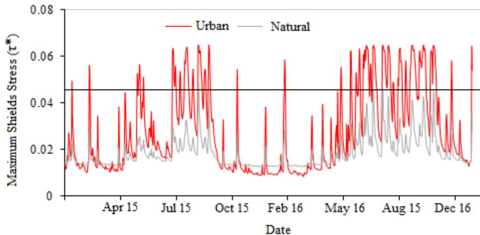
Figure 3 Daily maximum bed shear stress for the urban and natural reach for the study period. Horizontal black line indicates critical Shield stress,  $\tau_c^*$ .
