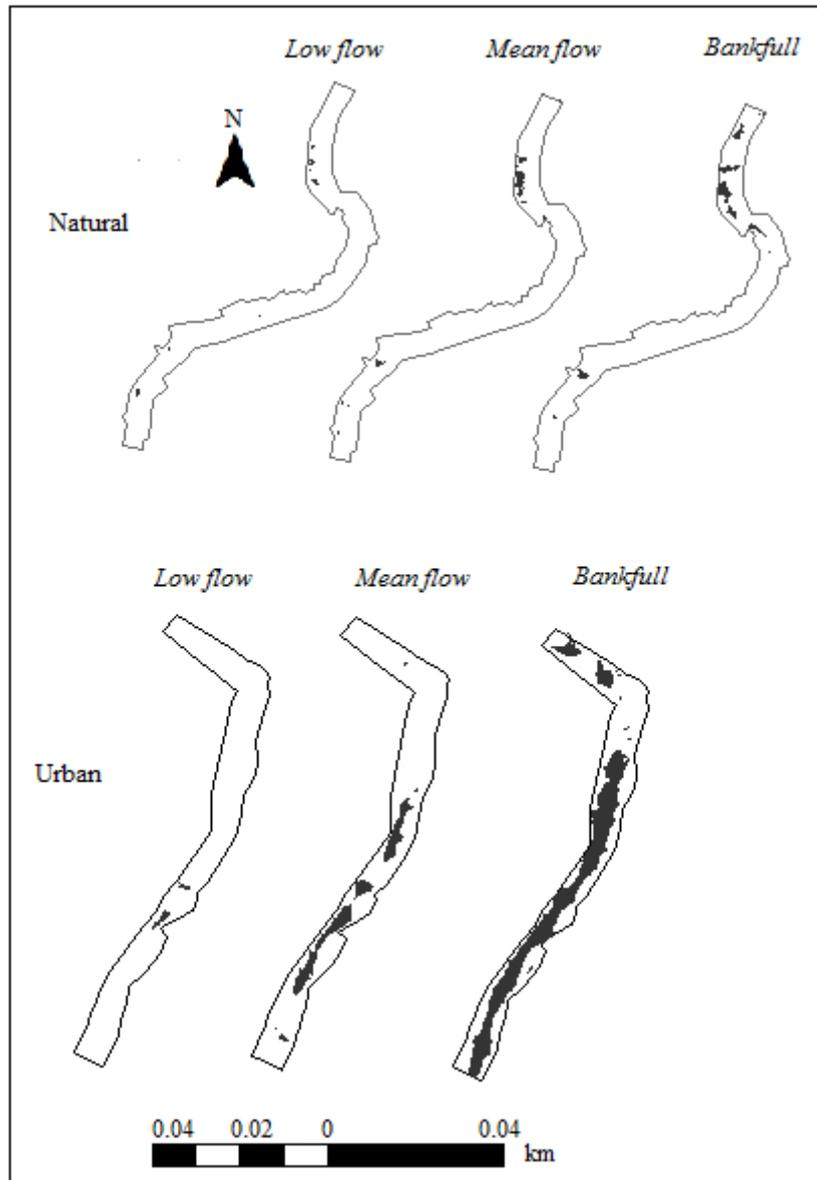
Figure 4. Planform maps of Shield stress pattern for low, mean and bankfull flow indicating spatial distribution of potential bed movement location as flow increases at each site. Shaded black represents area where Shield stress is above critical.
