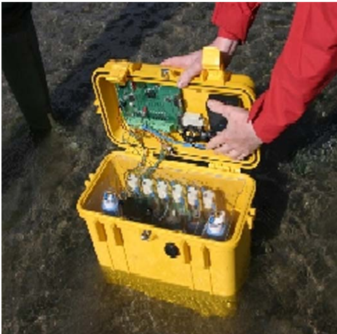
Fig. 4 One category of a sensor harnessed by SmartBay. This example measures phosphate levels
