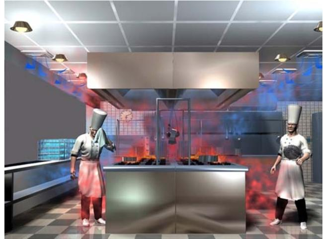
**Figure 7** *Mixing ventilation, supplying air through ceiling diffusers at the ceiling level.*
