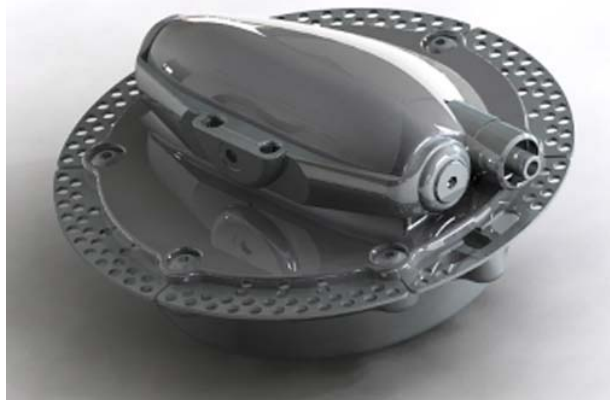
Fig. 1 The seventh-generation muscle energy converter (MEC) pictured from above. This device features a rotary cam mechanism that compresses an internal bellows as the outer armature is rotated upward (90 degrees max). Machined into the actuator arm is a semi-circular channel designed to accommodate a looped artificial tendon (CardioEnergetics, Inc.) that connects the muscle to the MEC. The device is placed through a window created in the chest wall by removing a 6.5-cm segment of one rib. The housing is anchored to the adjoining ribs using steel suture wound around a ring of perforated tabs extending 0.7 cm from the device periphery.
