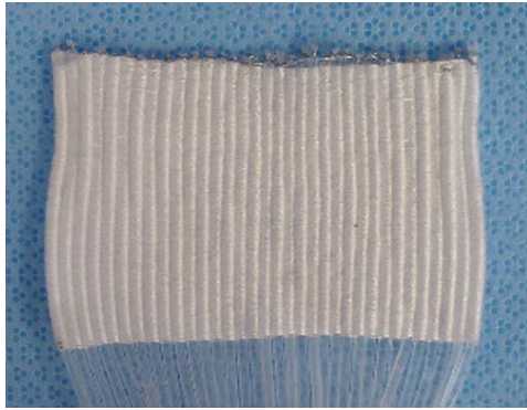
Fig. 3 Photograph of a prototype hydraulic contractile element formed from 34 thin-walled silicone tubes (0.147 cm ID, 0.193 cm OD) arranged in parallel and secured in tight approximation using fine polyester fiber. The fiber is woven in an over-and-behind fashion across the entire width of the assembly to a height of 4.3 cm so that a solid fabric surface is created. This allows the tubing to collapse completely when empty and to assume a full circular cross section when inflated. This also provides a means to support the tubing walls during high-pressure inflation while maintaining secure sidewall approximation throughout the contraction cycle.
