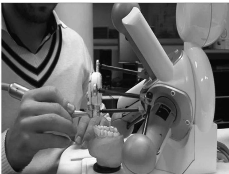
Figure 4. View of a haptic force feedback. The device is composed of three articulated branches, attached in parallel to a grasping tool that gives kinematic feedback on all degrees of all axes.
