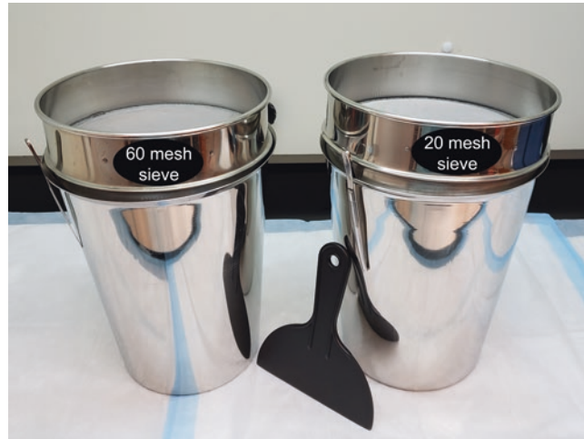
Fig. 4 Example of stainless steel buckets paired with stainless steel sieves for sieving stool samples. Note the use of forceps to create a break at the interface between the buckets and the sieves (prevents vapor seal/lock during sieving, otherwise sample spattering can occur when lifting the sieves). If buckets have pouring spouts, the forceps are not needed. Disposable plastic spatula for assisting sieving of stool samples (along with water or saline spray bottles)
