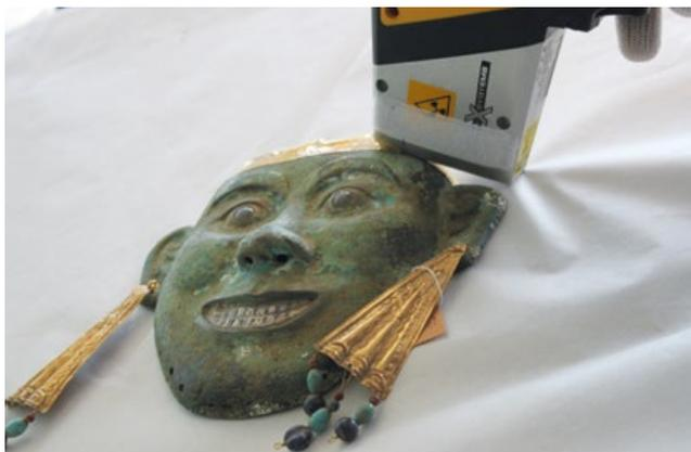
Fig. 2 | XRF-analysis carried out on the object CE01099.
