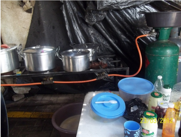
Figure 1: LPG stoves used in street cooking enterprises, Alexandra Township
