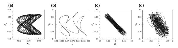
Fig. 8 Force diagrams for selected values of Re on the route to chaos:  $C_x - C_y$  diagram for Re = 220 (a) and Re = 230 (b);  $C_y - C_z$  diagram for Re = 245 (c) and Re = 270 (d)
