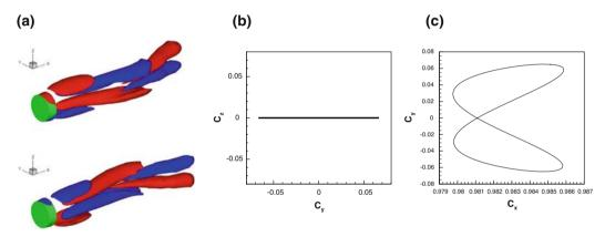
Fig. 5 Periodic mode with reflectional symmetry and zero mean lift (or "Zig-Zag" mode) for Re = 216. a Iso-levels of the streamwise vorticity in the plane located at x = 0.5, b  $C_y - C_z$  diagram, c  $C_x - C_L$  diagram
