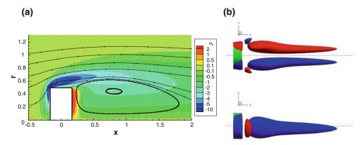
Fig. 1 Steady flow regimes: a axisymmetric flow for Re = 150 depicted by azimuthal vorticity (*colors online*) and streamlines, b non-axisymmetric steady state (SS) for Re = 165 depicted by iso-surfaces of the streamwise vorticity (two orthogonal views)
