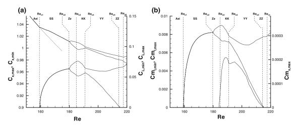
Fig. 6 Variations of force coefficients (a) and torque coefficients (b) in the range  $Re \in [150, 220]$
