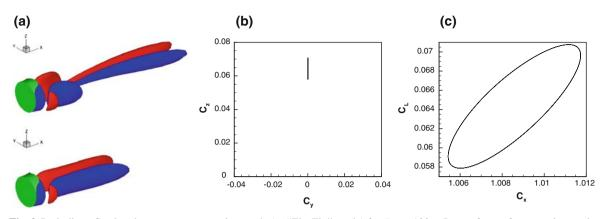
Fig. 2 Periodic, reflectional-symmetry-preserving mode (or "Zig-Zig" mode) for Re = 182. a Iso-surfaces of streamwise vorticity (at two time instants of the cycle corresponding to the maximum and the minimum of the lift force, respectively), b  $C_y - C_z$  diagram, c  $C_x - C_L$  diagram
