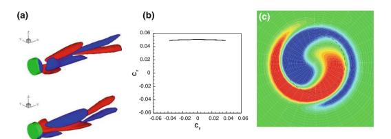
Fig. 4 Periodic, reflectional-symmetry-breaking mode (or "Yin-Yang" mode) for Re = 195. a Iso-surfaces of the streamwise vorticity at two instants, b  $C_y - C_z$  diagram, c iso-levels of the streamw vorticity in the x = 0.5 plane
