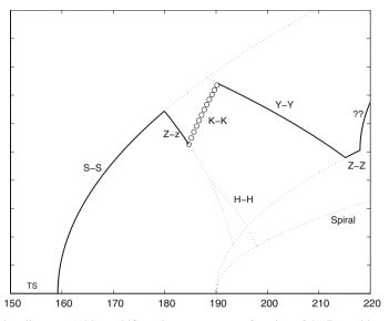
Fig. 7 Theoretical bifurcation diagram. Arbitrary bifurcation parameter as function of the Reynolds number. Full (resp. *dashed*) lines represent stable (resp. unstable) branches; *circles* represent the quasi-periodic pulsating "Knit-Knot" branch
