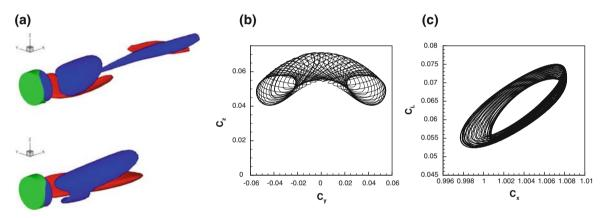
Fig. 3 Quasi-periodic pulsating mode (or "Knit-Knot" mode) for Re = 187. a Iso-surfaces of the streamwise vorticity at two instants of time, b  $C_y - C_z$  diagram (the end of the time series is represented with a *thick line*), c  $C_x - C_L$  diagram
