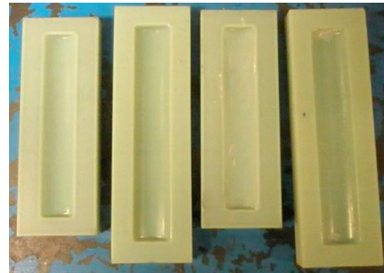
Fig. 9. Finished cavities: as printed, hot-pressed, scraped/polished, coated.
